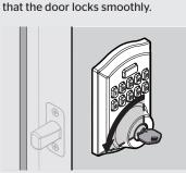
Turn the key 180° to retract the latch. Ensure that the door unlocks smoothly.
