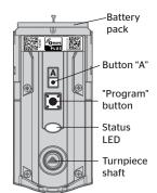
Note: When the cover is removed, the turnpiece shaft can be used to manually lock and unlock the door.
