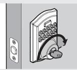
Close the door. Insert and rotate the key to lock the door. Ensure
