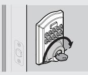
If your door does not lock and unlock smoothly, make sure you replaced your previous latch and strike with those supplied in the box. If you still experience locking errors, complete the troubleshooting steps at http://bit.ly/HC620jam or call Kwikset Support: 1-866-863-6584
